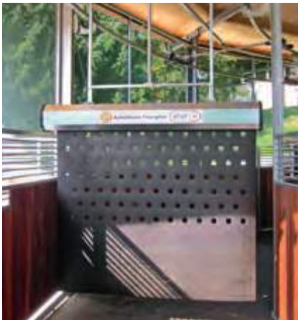
Retractable gates simplify and facilitate cleaning in the horse walker.
