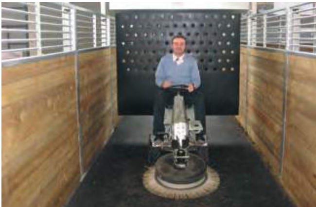
Combination of rubber floor and retractable gates make mechanical cleaning possible.
